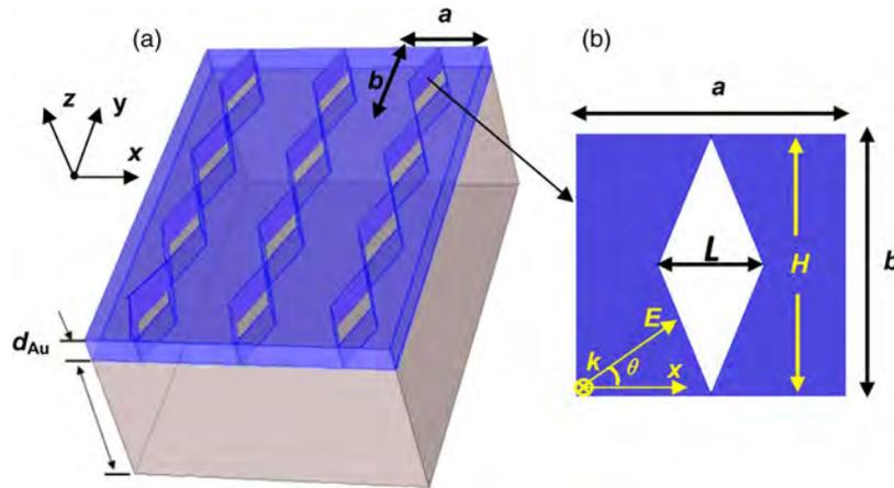
Fig. 1. (a) Proposed paradigm structure consisting of Au patterned film with thickness  $d_{Au}$  resting on a  $d_{sub}$  thick substrate. (b) The unit cell of the structure is magnified and depicted on the right panel (top view), with the associated geometric features.
