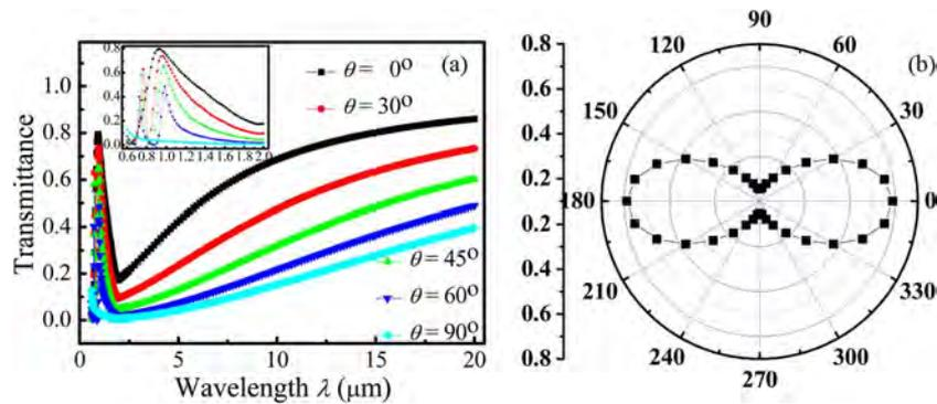
Fig. 2. (a) Transmission spectra of the diamond-shaped nanohole arrays irradiated by light with polarizations of  $\theta = 0^\circ, 30^\circ, 45^\circ, 60^\circ, 90^\circ$ . Inset figure is the transmittance spectra of the wavelength ranging from  $0.6 \mu\text{m}$  to  $2.0 \mu\text{m}$ . (b) Polar plot of the transmittance of the diamond-shaped nanohole arrays at  $\lambda = 10 \mu\text{m}$  with different polarizations.
