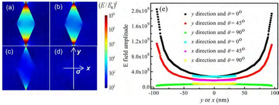
Fig. 3. (a)–(d) Contour profiles of the normalized  $|E_z|$  fields of the diamond-shaped nanohole arrays at different polarizations at  $\lambda = 10 \mu\text{m}$ . (a)  $\theta = 0^\circ$ . (b)  $\theta = 30^\circ$ . (c)  $\theta = 60^\circ$ . (d)  $\theta = 90^\circ$ . (e) Electric field amplitude along the diagonal lines ( $x$  and  $y$  directions) under irradiations at  $\lambda = 10 \mu\text{m}$  with different polarization angles.
