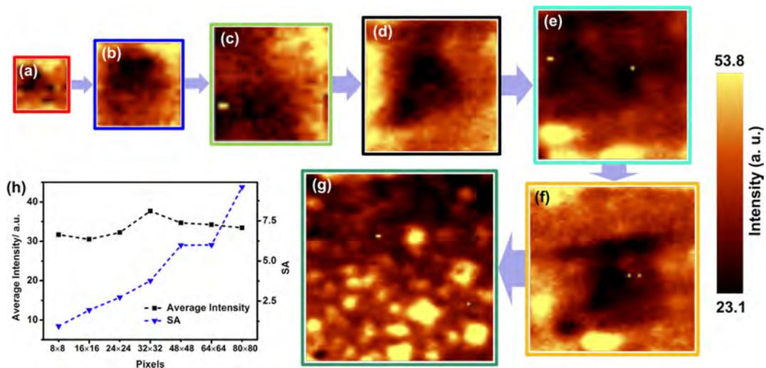
**Fig. 8.** The Raman mappings of 10 μM CV on Substrate-250 with varied area and pixels. (a) 8 × 8 pixels (3.5 × 3.5 μm<sup>2</sup>); (b) 16 × 16 pixels (7.5 × 7.5 μm<sup>2</sup>); (c) 24 × 24 pixels (11.5 × 11.5 μm<sup>2</sup>); (d) 32 × 32 pixels (15.5 × 15.5 μm<sup>2</sup>); (e) 48 × 48 pixels (23.5 × 23.5 μm<sup>2</sup>); (f) 64 × 64 pixels (31.5 × 31.5 μm<sup>2</sup>); (g) 80 × 80 pixels (39.5 × 39.5 μm<sup>2</sup>); (h) the average intensity and SA as a function of mapping area.
