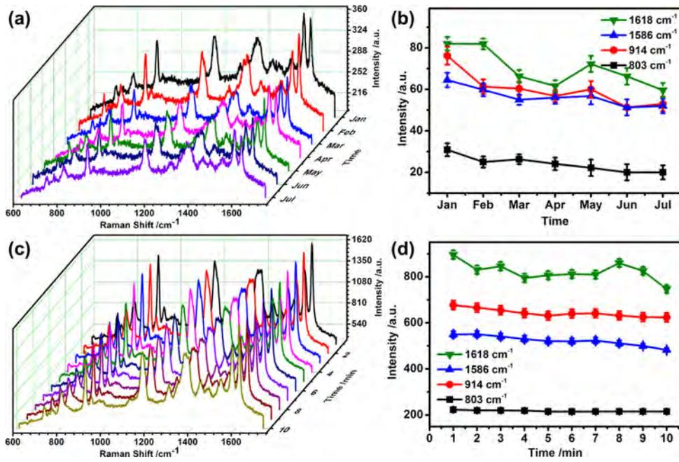
**Fig. 6.** (a) The raw Raman spectra of 1 μM CV on Substrate-50 collected at different time; (b) the variation of Raman intensity at different time; (c) the raw Raman spectra of 1 μM CV on Substrate-250 collected under 215 μW laser exposure; (d) the variation of Raman intensity at different time under 215 μW laser exposure.
