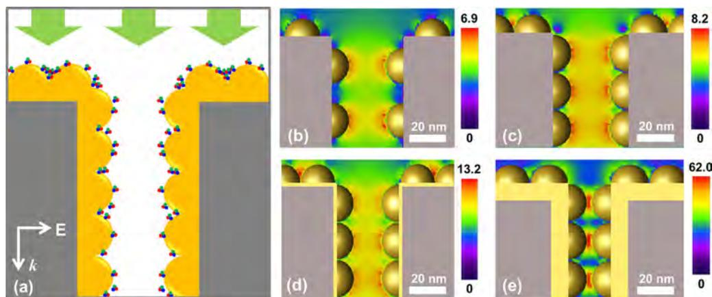
**Fig. 5.** The FDTD simulations for MnO<sub>2</sub>/Au hybrid nanowall film; (a) the model of MnO<sub>2</sub>/Au hybrid nanowall film for simulation; (b)–(e) FDTD simulations of the electric field distribution in cross-section view of MnO<sub>2</sub>/Au hybrid nanowall film with varied gold thickness.
