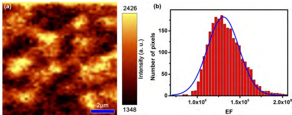
**Fig. 7.** (a) The Raman mapping of 1 μM CV on Substrate-200; (b) the histogram of EF distribution in mapping area.
