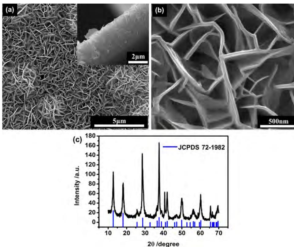
**Fig. 2.** (a) The top-view SEM image of MnO<sub>2</sub> nanowall film on silicon wafer, the inset is the cross-section view of the MnO<sub>2</sub> nanowall film; (b) the high magnification SEM image of the MnO<sub>2</sub> nanowall film; (c) the XRD pattern of the MnO<sub>2</sub> nanowall film.
