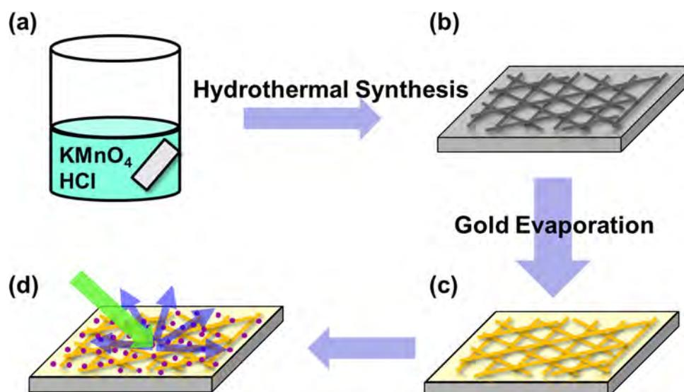
Fig. 1. Schematic illustration of overall experimental process.
