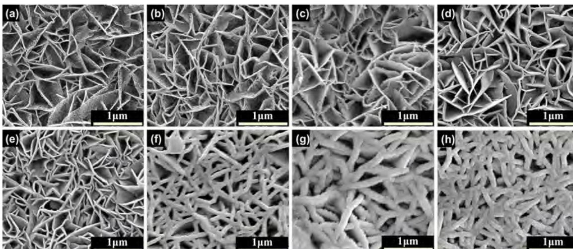
**Fig. 3.** The top-view SEM images of MnO<sub>2</sub>/Au hybrid nanowall film. (a) Substrate-5; (b) Substrate-10; (c) Substrate-15; (d) Substrate-25; (e) Substrate-30; (f) Substrate-100; (g) Substrate-200; (h) Substrate-250.
